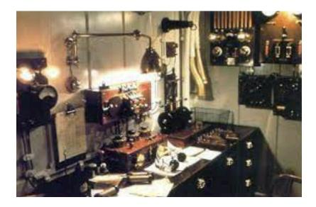
These first radio transmitters, spark gap transmitters, were used as wireless telegrams. They worked by charging and discharging a capacitor and shooting a spark across a gap producing radio waves over a range of different frequencies and amplitudes. The system could not send audio messages, but rather a code, such as Morse code, when the operator switched the transmitter on and off. However, these pulses of radio waves caused a lot of interference making complex communication very difficult.
